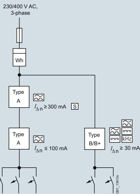
When configuring and installing electrical installations, electrical loads that can generate smooth DC residual currents in the event of a fault must be assigned a separate electrical circuit with a universal current-sensitive residual current protective device (type B) (see configuration example).
