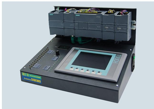
The training case is used to realistically practice the programming, operating and commissioning of SIMATIC S7-1200 controllers.
