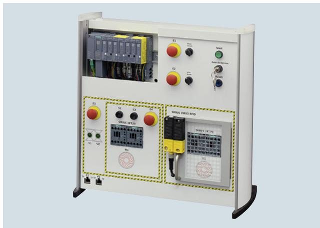
The training case is used to simulate realistically periphery to practice the programming, operating and commissioning of failsafe SIMATIC S7-1500 controllers within TIA Portal.
